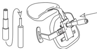
2 Slide the 3-piece plastic sleeve over the cylinder. (The sleeve should telescope from the smallest segment over the cylinder head to the largest at its base.) Then, insert cylinder into the hole in the mechanism as shown.
