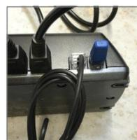
The collision detection dongle has the ability to interrupt the power to the desk.
