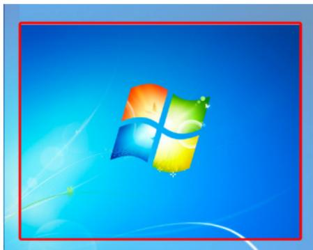
A red border will appear on the Extended screen that will show the size of the new Windows Desktop. Use the horizontal and vertical + and - buttons to manually adjust the size to properly fit the screen.
